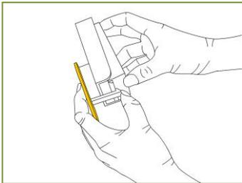
🐾 Hold both sides of the transmitter button and slide the transmitter out of the housing, bottom first.
