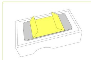
🐾 With the **inside arrow pointing upward**, press the housing firmly onto the wall, just **above the mark**.
